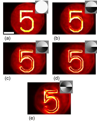
Fig. 2. Contrast modifications emulated by means of the SLM device being addressed with fractional spiral phase functions (fractional Riesz transform) of fractional coefficient (a)  $l=0$ , (b)  $l=0.4$ , (c)  $l=0.8$ , (d)  $l=1.0$ , (e)  $l=2$ .
