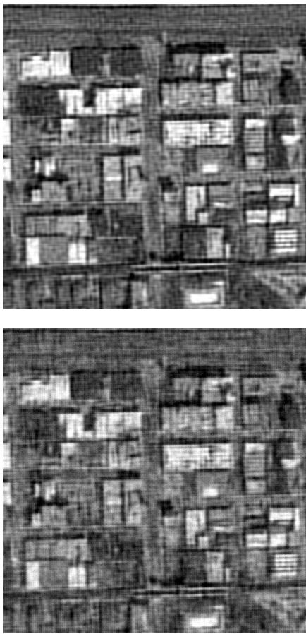
Fig. 5. Top: A 512x512 crop of a 2048x2048 image with a sparsity of 2%. Bottom: Image after running the proposed sFFT algorithm. The PSNR is 23.3dB when compared to the original sparse image.
