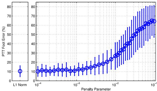
Fig. 5. While the standard deviation of the  $PTT_f$  is higher than that of the RMS difference, the general trend is the same at a USR of 16. As the penalty parameter decreases, the accuracy increases.
