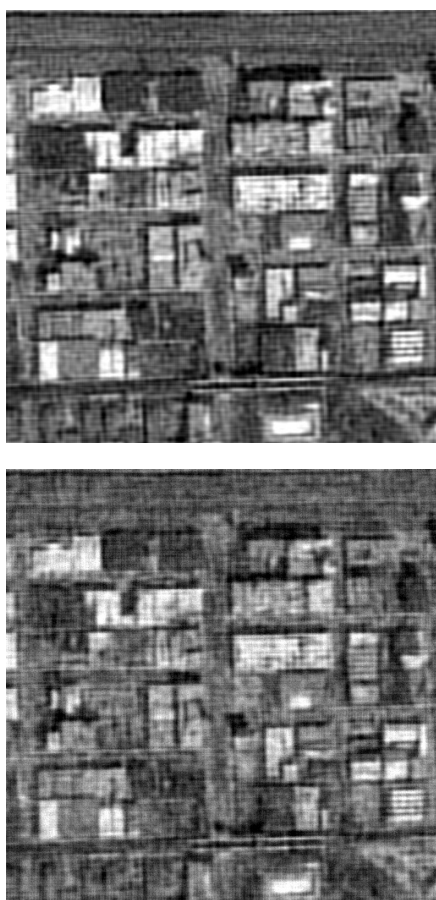
Fig. 5. Top: A 512x512 crop of a 2048x2048 image with a sparsity of 2%. Bottom: Image after running the proposed sFFT algorithm. The PSNR is 23.3dB when compared to the original sparse image.
