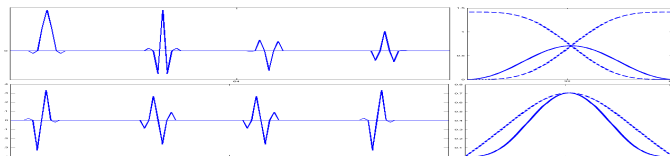
Fig. 1. Top:FB generating tight frames: impulse and magnitude responses derived from quadratic quasi-interpolating spline. Bottom: analysis and synthesis band-pass filters for semi-tight frame
