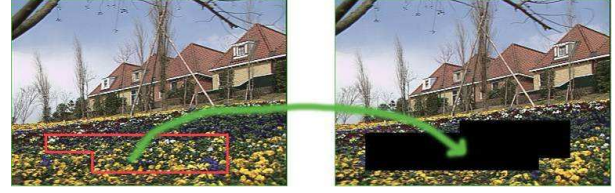
Fig. 4. The Motion Model is Used For Warping the Texture From The Key Frame to Texture Frame.
