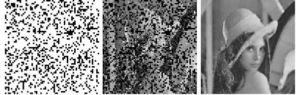
Figure 2. Lena attractor 4x4 range block size, decoded in the case that the bottom half of the fractal code is missing. Seed image is black. POCS scheme [11]
