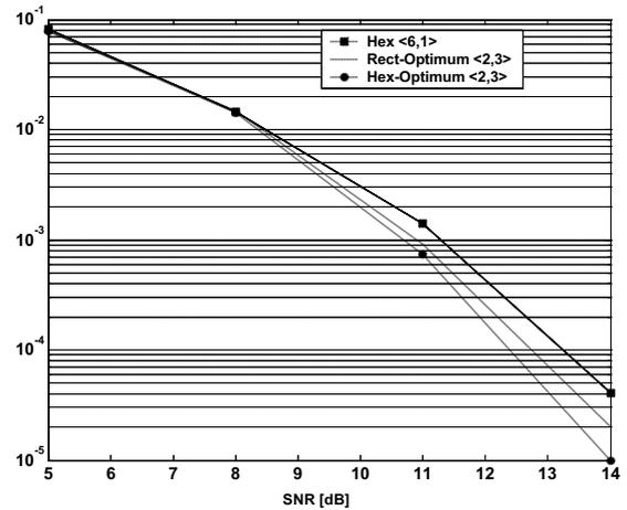
Fig. 7. OFDM system performance with velocity  $v=100$  Km/h,  $\tau_{\max} =100$ ns,  $dp=16.6\%$
