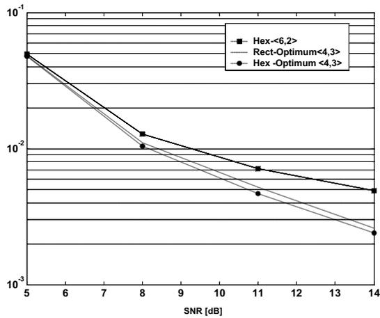
Fig. 4. OFDM system performance with velocity  $v=60$  Km/h,  $\tau_{\max}=50$ ns, and  $dp=8.33\%$
