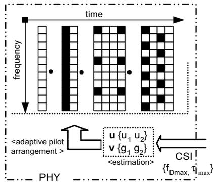
Fig.3. Description of different pilot system locations
