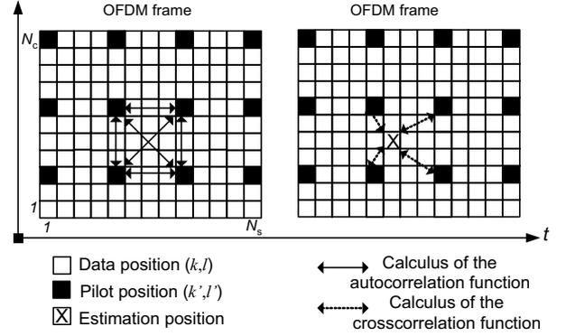
Fig. 2. A rectangular pilot spacing with  $N_c=11$ ,  $N_s=13$ ,  $N_t=5$ ,  $N_f=5$  and  $\text{tap}=4$ .
