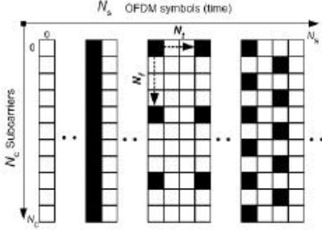
Fig. 1. Time-frequency pilot arrangement in an OFDM frame.
