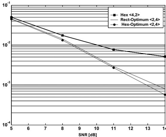
Fig. 6. OFDM system performance with velocity  $v=60$  Km/h,  $\tau_{\max}=100$ ns, and pilot density  $dp=12.5\%$ .
