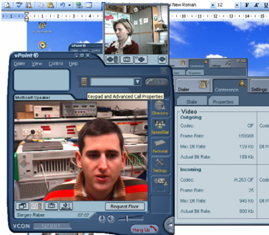
Fig. 7 An interactive multicast stream from FHI is displayed in the large video screen (bottom). After requesting floor by clicking on the "request floor" button, the local video and audio streams of TUG (top) were sent via UDPTunnel to FHI and then transmitted via satellite to remote attendees.
