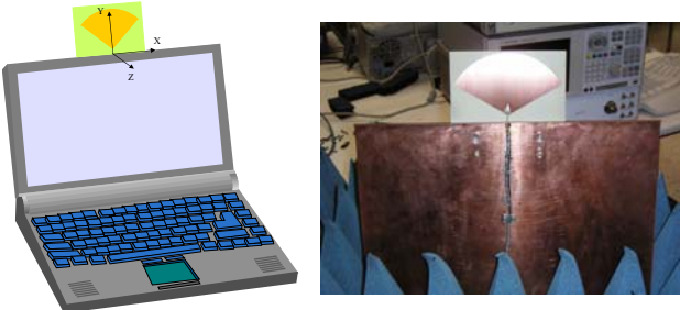
Fig. 6a/b. Antenna installation concept and prototyping including the metallization of the portable PC back and the antenna.
