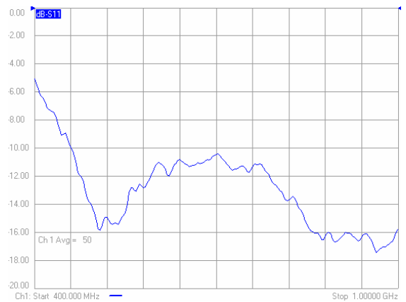
Fig. 4. Measured insertion losses for the circular dipole antenna.
