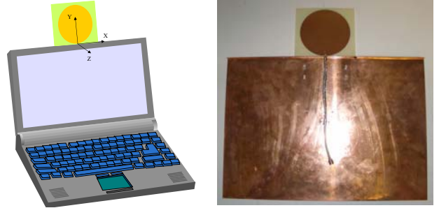
Fig. 3a/b. Antenna installation concept and prototyping including the metallization of the portable PC back and the antenna.
