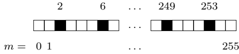
Fig. 1. Pilot pattern defined by (1) for block length M = 256 and J = 60 pilot symbols.
