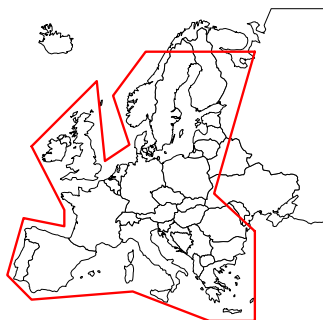
Figure 3: Typical S-band service downlink coverage
