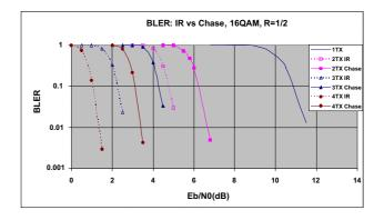
Fig. 7: HARQ type 2 residual BLER: IR vs. CC comparison.
