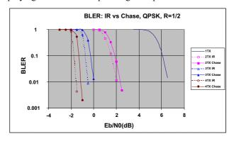
Fig. 6 HARQ type 2 residual BLER: IR vs. CC comparison.
