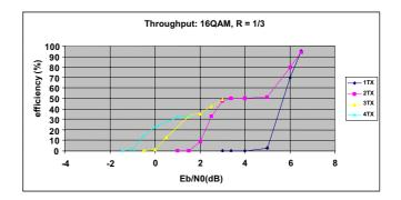
Fig. 4: HARQ type 1 throughput efficiency: maximum throughput per user: 1878kbit/s.
