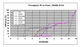
Fig. 9: HARQ type 2 throughput efficiency: IR vs. CC comparison, maximum throughput per user: 4284kbit/s.
