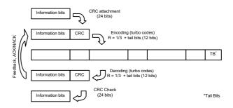
Fig. 1: Data flow graph for HARQ type 1 scheme
