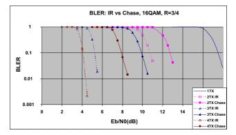
Fig. 8 HARQ type 2 residual BLER: IR vs. CC comparison.
