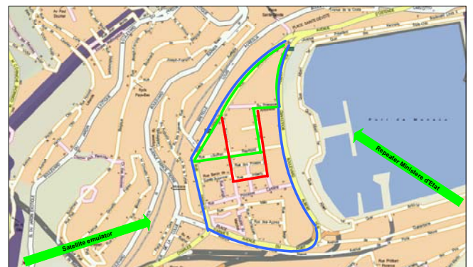
figure 2: General direction of satellite emulator antenna (left arrow) and repeater antenna (right arrow). Main urban test drives are indicated in blue, red and green.
