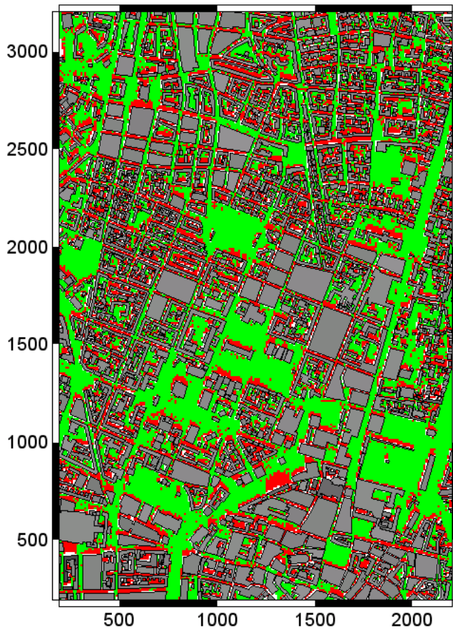
Fig. 4. Coverage in Munich for pure satellite network.
