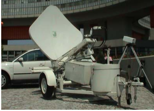
Figure 1. Mobile Satellite Earth Station connected with FSO
