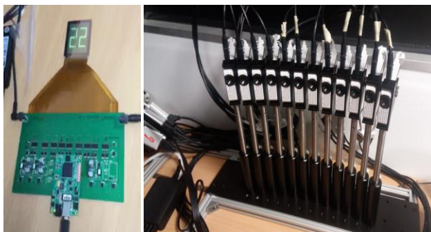
Figure 6 SMV prototypes: Left-1 kHz OLED, Right-36-view
