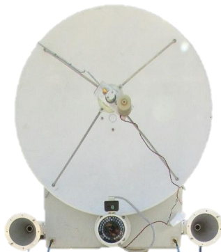
Fig. 4. Image of placement of transmitter reflector and two receiver antennas
