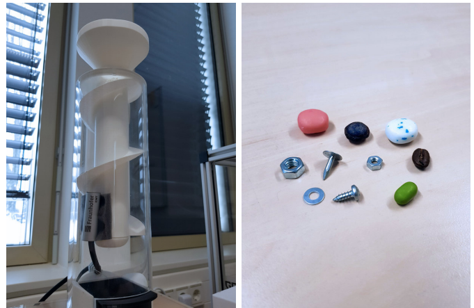
Fig. 3. Tube with slide and mounted external microphone (left). Bulk material (right).
