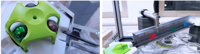
Fig. 2. Launch pad with all ball types (left). Slide with mounted microphone (right).
