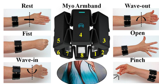
Fig. 2. Myo armband and the gestures recognized in this paper.
