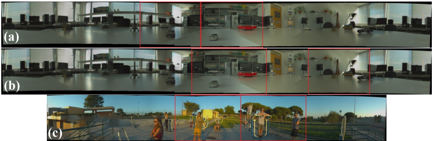
Figure 7. Three light field panoramas: depth plane extracted with (top) slope = -0.05 , (middle) slope = 0.6 and (bottom) slope = 0.15 .
