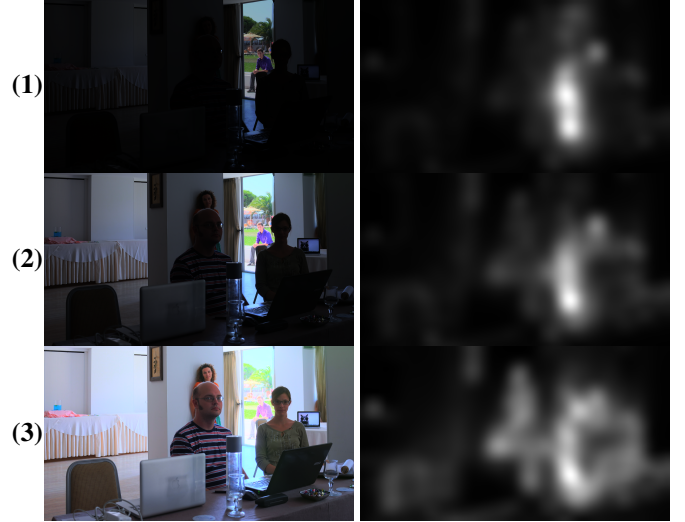
Fig. 2: (1) Tone mapped under exposure image and corresponding saliency map, (2) Tone mapped proper exposure image and corresponding saliency map, (3) Tone mapped over exposure image and corresponding saliency maps.
