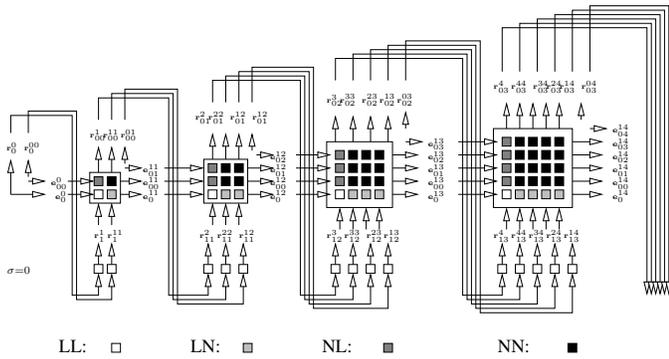
Fig. 11. The block structure of the nonlinear Schur parametrization of a 4-th order stationary stochastic process ( $n = 4$ ).
