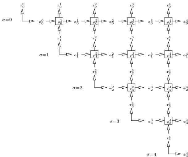
Fig. 3. Linear Schur parametrization of a 2-nd order nonstationary stochastic process ( $n = 4$ ).
