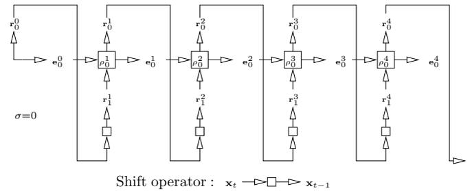
Fig. 4. Linear Schur parametrization of a 2-nd order stationary stochastic process ( $n = 4$ ).
