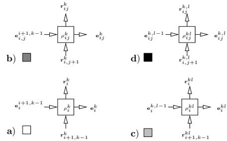
Fig. 6. Elementary linear/nonlinear hyperbolic rotations: a) LL (Linear-Linear), b) NL (Nonlinear-Linear), c) LN (Linear-Nonlinear), d) NN (Nonlinear-Nonlinear).
