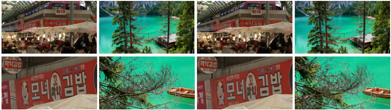
Fig. 2. Images from from DIVK2K Val set with low and high M_h values. Top row from left to right: Image 831 blurred by 11x11 box-filter; Image 807 blurred by 11x11 box-filter; Image 831 linearly interpolated by a factor of 4 after low-pass filtering by 4x4 box-filter and downsampled by 4; Image 807 linearly interpolated by a factor of 4 after low-pass filtering by 4x4 box-filter and downsampled by 4. Bottom row from left to right: The first two images are zoomed restored patches corresponding to the red window from the blurred images on the top; The last two images are the corresponding patches from the output of the SISR network. Note that M_h for Image 831 is 948 and its PSNR for restoration is 35 dB and for SISR is 29.3 dB. The M_h for Image 807 is 8499, and its PSNR for restoration is 24.6 dB and for SISR is 19.8 dB, which demonstrate that M_h values correlate well with PSNR. Observe that both restoration and SISR results for Image 831 do not contain visual artifacts, while there are annoying artifacts in both restoration and SISR results for Image 807 near the tree branches.
