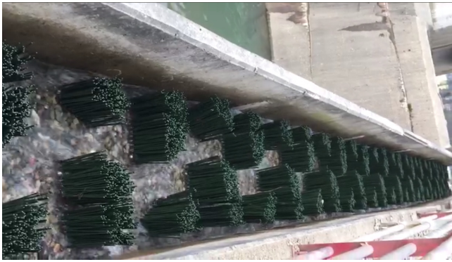
Fig. 1. Brush based fishway model used in experiments.
