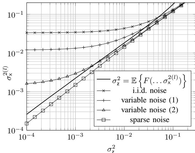
Fig. 3. “Exit-plot”: the evolution of  $\sigma_z^2$  and  $\sigma_x^{2(l)}$ , estimated with State Evolution for a subsampling factor  $\rho = 0.6$  and SNR = 10dB.
