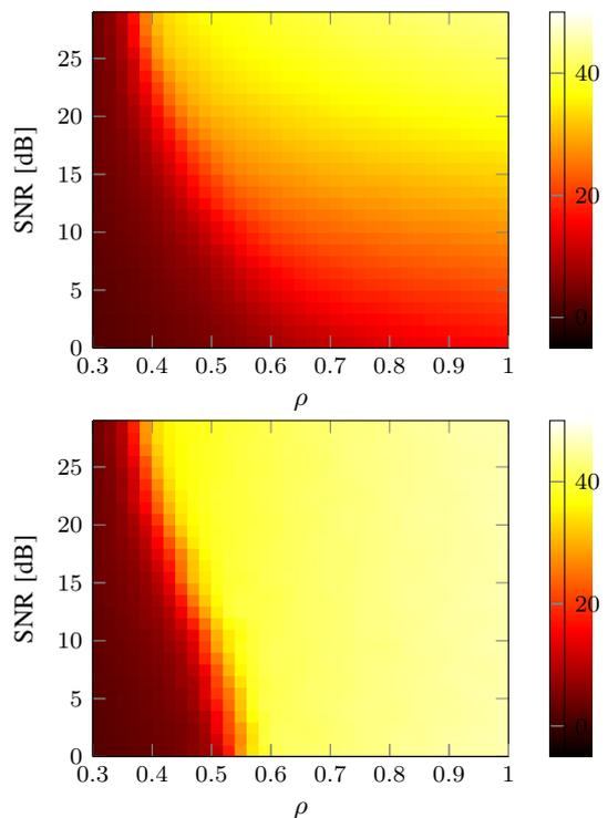
Fig. 5. Recovery SDR [dB] (color coded) vs. subsampling ratio  $\rho$  and noise SNR. AMP-VN with variable noise (variant 2, top) and sparse noise (bottom).
