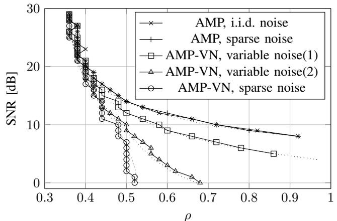
Fig. 1. Phase transition for Bernoulli-Gauss prior. The recovery SDR is larger than 10dB northeast of the curve. The dotted lines are the result of State Evolution estimation of the 10dB recovery SDR threshold of the associated curve. The SNR on the y-axis is the average measurement noise according to (43),  $\rho$  is the undersampling factor.
