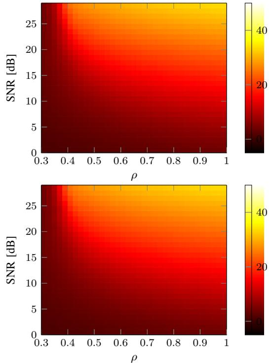
Fig. 4. Recovery SDR [dB] (color coded) vs. subsampling ratio  $\rho$  and noise SNR. Standard AMP with i.i.d. noise (top), with sparse noise (bottom).
