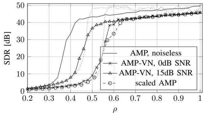
Fig. 2. Recovery SDR versus subsampling factor  $\rho$  for noiseless AMP and AMP-VN in presence of sparse noise. The "scaled AMP" plot is for comparison purposes only and explained above. The dotted curves are the result of State Evolution for AMP-VN at 15dB and 0dB SNR in presence of sparse noise. In the convergence region the predicted SDR deviates due to differing abortion criteria.
