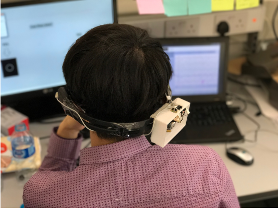
Fig. 2: The setup for the system. The EEG recording machine along with the synchronization circuit inside a three-dimensional (3D) printed enclosure. The thickness of the walls is less than 1mm making the total weight low and not affecting the balance of the headset
