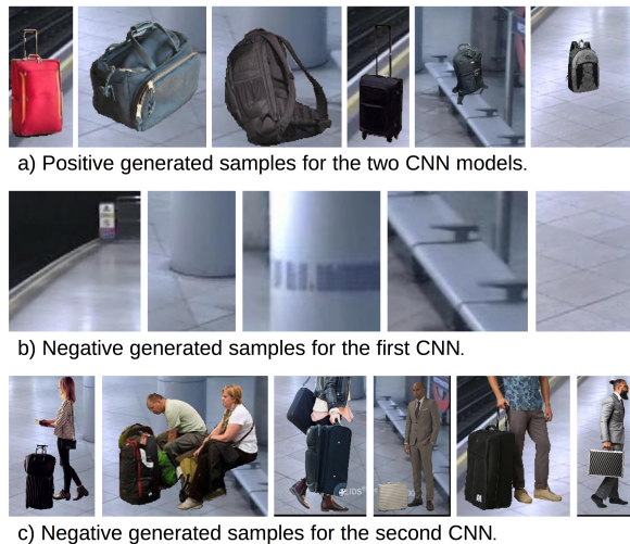
Figure 2. Realistic image samples generated by randomly sampling sub-images from the estimated background image (second row) and by superimposing luggage items (first row) or people standing by their luggage items (third row). These samples are used to fine-tune our convolutional neural networks for a particular scene. Best viewed in color.
