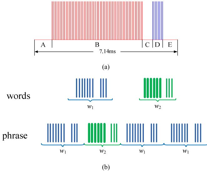
Fig. 1. An example of the hierarchical structure of “Mercury” radar signals
