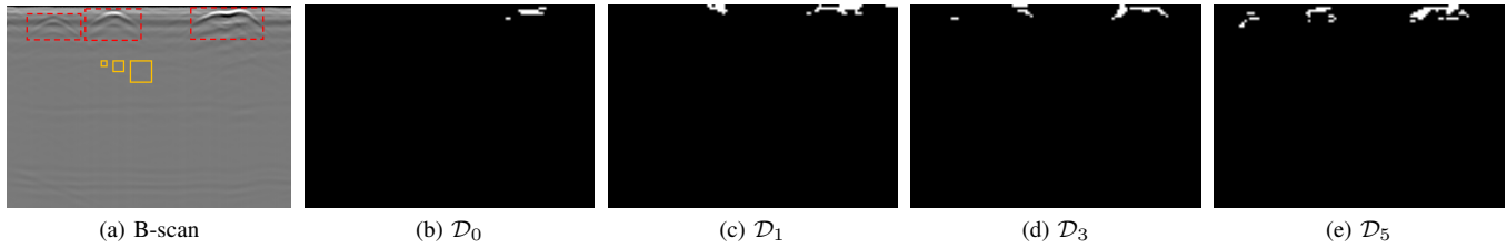
Fig. 3: Examples of detection masks obtained thresholding weights w_n according to \Gamma . White areas indicate patches detected as containing hyperbolic traces. (a) reference B-scan with three targets (dashed rectangles) and example of patches for B \in \{32, 64, 128\} ; (b) mask obtained for R = 0 ; (c) mask obtained for R = 1 ; (d) mask obtained for R = 3 ; (e) mask obtained for R = 5 .
