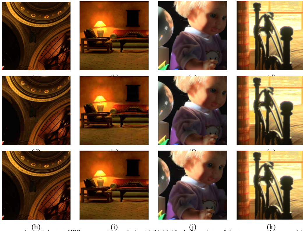
Fig. 3. Subjective comparison of the test HDR compression methods: (a)-(b)-(c)-(d) close-up shots of the tone-mapped images, (e)-(f)-(g)-(h) decoded tone-mapped images using JPEG XT, (i)-(j)-(k)-(l) decoded tone-mapped images using our method.
