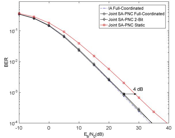
Fig. 3. BER Performance at the Small-cell System using QPSK modulation.
