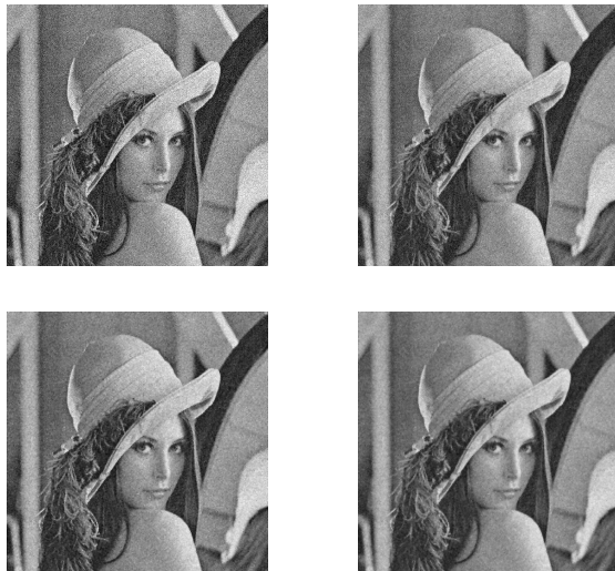
Fig. 5. From left to right top to bottom: noisy I ( \sigma = 25 , PSNR = 20.22, SSIM = 0.599), preprocessed I_P (PSNR = 22.88, SSIM = 0.687), denoised I_d (PSNR = 27.27, SSIM = 0.763) and denoised preprocessed I_{P,d} (PSNR = 28.49, SSIM = 0.812) Lena image.
