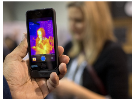
Fig. 1. Example of a consumer-level thermal camera 1 .
