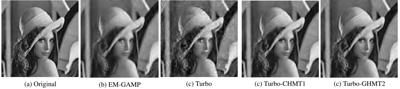
Fig. 6. Reconstruction with 30% CS observations of the 128 \times 128 lena image using various algorithms.
