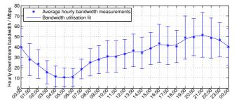
Fig. 8. Mean downlink bandwidth of Tiree network and fitted model.
