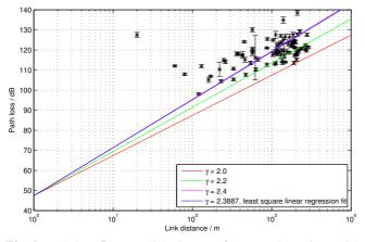
Fig. 5. Path loss L versus link distance d measured on Tiree, with linear approximations and a least squares fit.
