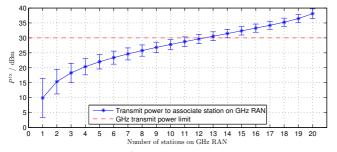
**Fig. 6.** Mean beliefs of  $\mathcal{P}_g^{tx}$  with standard deviation after BBN convergence to associate stations with the GHZ RAN.
