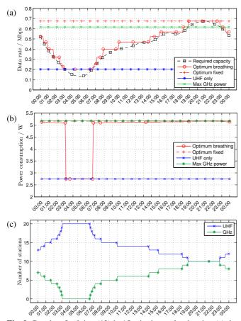
**Fig. 9**. Results of solving (12) in 15 min. intervals, showing (a) the required and offered capacity, (b) the total network power consumption and (c) the station assignment.
