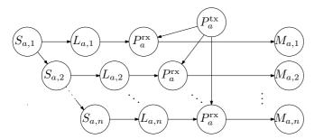
**Fig. 2.** BBN describing dependencies of distance, path loss, receive power and data rate.
