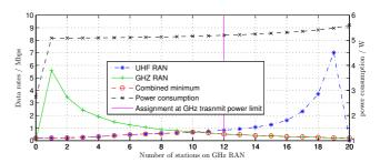
**Fig. 7.** Individual station capacity on each RAN and base station power consumption given possible valid RAN assignments.
