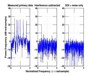
**Fig. 2.** Simulated NQR-signal with interference containing six damped sinusoids, randomly positioned. The left figure shows the measured primary data, whereas the middle figure shows the primary data after EPIC has removed the interference. The right figure shows the simulated NQR-signal without interference.
