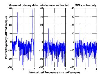
**Fig. 1.** Simulated NQR-signal with interference containing two sinusoids, one of which is on top of the NQR-signal and one which is randomly positioned. The left figure shows the measured primary data, whereas the middle figure shows the primary data after EPIC has removed the interference. The right figure shows the simulated NQR-signal without interference.
