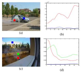
**Fig. 3.** (a)-(b) Variation of spatio-temporal energy for a block containing i) smoke (red block and line) and ii) a moving smoke colored object i.e. car (blue block and line), (c)-(d) variation of spatio-temporal energy for a block i) at the centre of smoke (red block and line), ii) at the edge of smoke (green block and line) iii) without smoke but with clouds (blue block and line).
