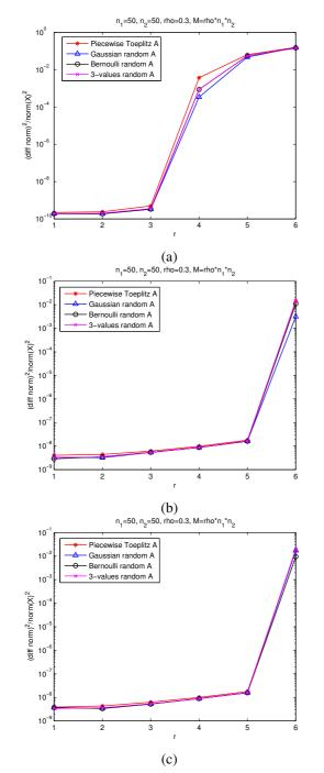
Fig. 2. Simulation results (a) using cvx toolbox to minimize the nuclear norm of **X** (b) using Alternating Least-Squares (ALS) algorithm (c) using Directional-ALS algorithm.
