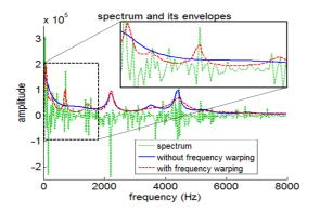
**Fig. 3**. Comparison of the envelopes. The green dotted line shows the spectrum of the input. The blue solid line and the red dashed line respectively indicate its envelopes extracted using linear prediction and the proposed method. The LP order of the envelopes was 16.
