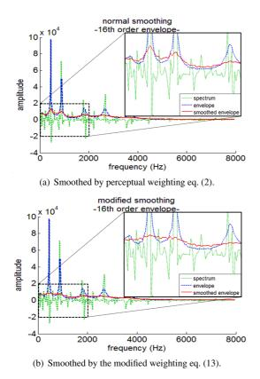
**Fig. 5**. The resolution-warped envelope smoothed by each method. The blue dashed line and the red solid line respectively indicate the envelope before and after smoothing. The LP order of the envelopes was 16.
