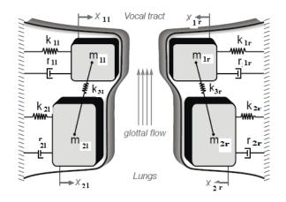
Fig. 1. Two-mass model of vocal folds [8].
