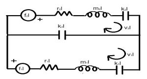
Fig. 2. Electromechanical equivalent circuit of vocal folds.
