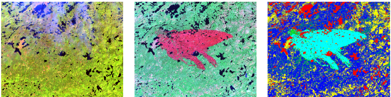
Figure 3. Landsat5-TM image pre-event; Landsat5-TM image post-event. Classification of post-event data ISOdata, 5 classes
