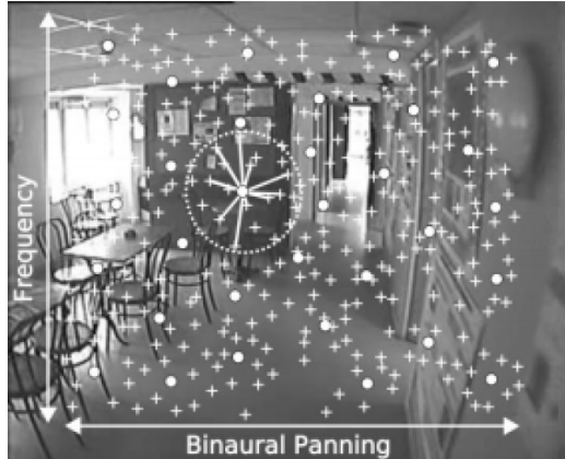
Figure 3: Example of retinal encoding applied to a gray-scaled image according to B. Durette. Crosses are pixels p used for the calculation. Filled circles are centers of the receptive fields.
