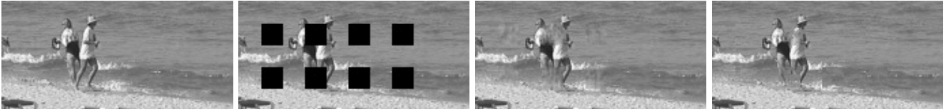
Fig. 2. Original image (first column); corrupted image (second column), PSNR=13.2 dB ; image recovered using the algorithm in [3] (third column), PSNR=20.59 dB ; image recovered using the proposed algorithm (last column), PSNR=20.65 dB.
