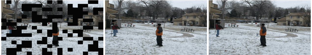
Fig. 3. Image with 50% of blocks are lost (first column), PSNR=9.01 dB; image recovered using motion compensation (second column), PSNR=28.26 dB; image recovered using the proposed algorithm (third column), PSNR=32.23 dB.
