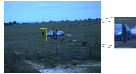
Fig. 8. the HOG detector fails to detect one of the pedestrians in a visual image. Using motion plus context, area is zoomed into and HOG now detects pedestrian.
