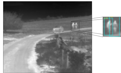
Fig. 9. The HOG detector fails to detect both of the pedestrians in a thermal image. Using motion plus context, the area is zoomed into and HOG now detects both pedestrians.
