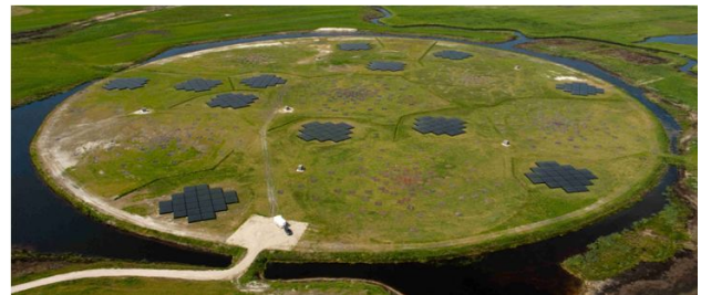
Fig. 1. LOFAR superterp. Core of the radio telescope located in Exloo, the Netherlands. LOFAR is composed of 4224 low band antennas (LBA, 30-80MHz) and 2496 high band antenna tiles (HBA, 120-240MHz), distributed over all Europe.
