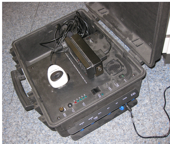
Fig. 1. Motorola's CM 5000 radio station, as used in the experiments
