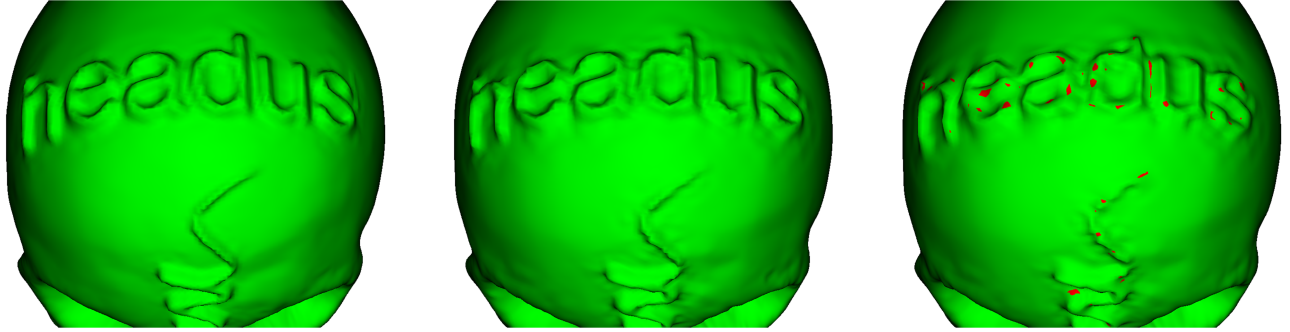
Figure 2. Visual comparison between the original Skull mesh model (left), the decoded version when employing the L-infinite driven SIM codec (center) and the L-2 driven SIM codec (right) at a target MAXAD of 2.1% of the bounding box diagonal corresponding to a rate of 0.607 bpv.
