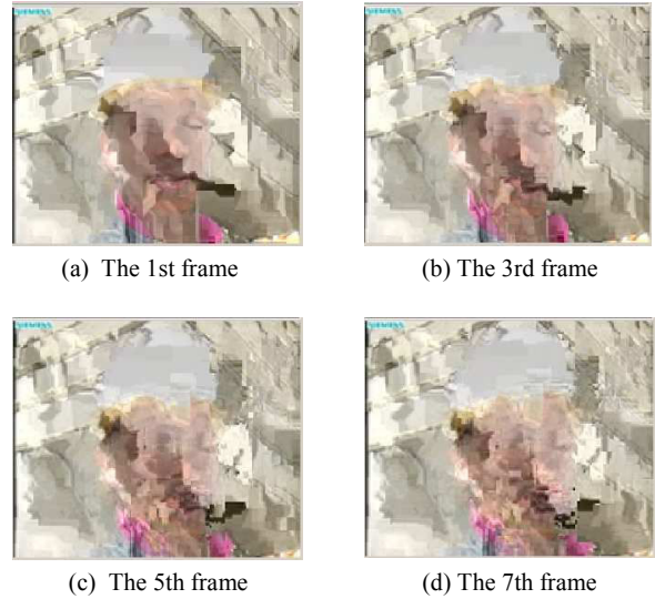
Fig. 6. The first few decoded frames of ‘foreman’ encoded in the baseline profile, with QP=18 and encrypted by IPM+IEMV.
