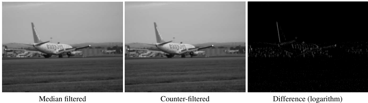
Fig. 3. An example of median filtered image and its counter-filtered version. As visible in the difference (logarithm is taken to enhance visibility) between the two, filtering mostly affects regions with higher variance, resulting in a perceptual high fidelity.
