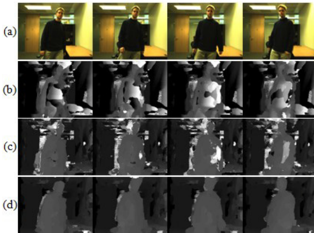
Fig. 5. Disparity map for “Jamie1”; (a) Left frames; (b) LASW; (c) Cost-filter; (d) Our method.
